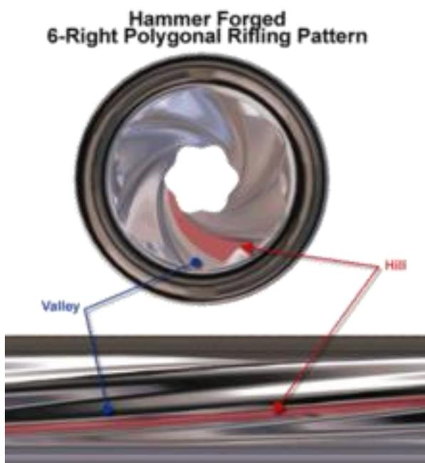
The diagram shows what a clockwise spin would look like by comparing a view down the barrel (top) and a cross section lengthways (bottom). The diagram uses more colloquial language for describing the components of the rifling, “Hills” (grooves) and “Valleys” (landings).
